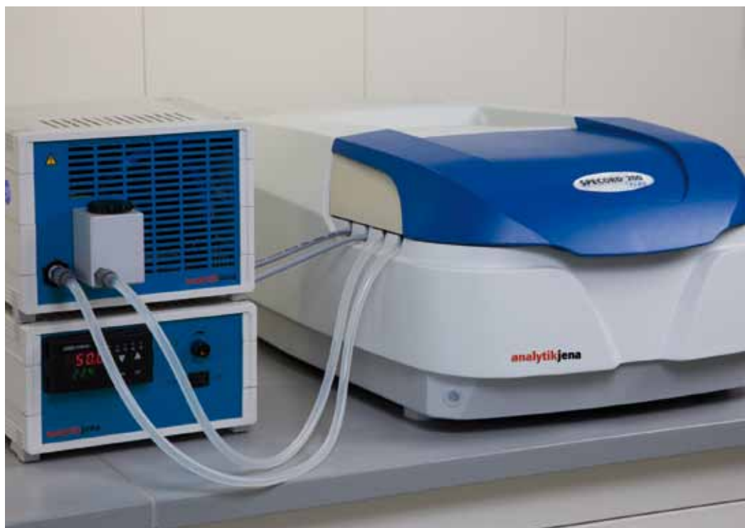
Temperature control via Peltier element
